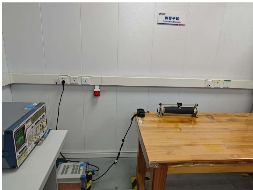
Conducted Emission at The Mains Terminals Test
