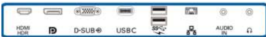
I/O back panel connector diagram
