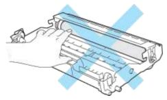
7. Clean the primary corona wire inside the drum unit by gently sliding the blue tab from right to left several times. Return the blue tab to the Home position before reinstalling the drum unit and toner cartridge assembly.
