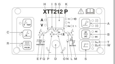
Arc force can be adjusted from 0-10, Arc force prevents the electrode from sticking during welding by surging the welding current if the arc voltage falls.
