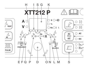
It is possible to use the pulse function with both AC and DC TIG welding Power Pulsing can give significant advantages on thinner material to control heat and penetration.
