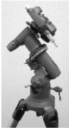
Figure 2-17 Dec. Lock Knob on top of Dec. circle & R.A. Lock Knob on top of R.A. circle
