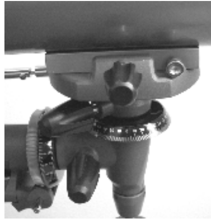
Figure 2-18 Mounting Knob & Safety Screw in the dovetail bracket Shown is the 114 EQ telescope tube
