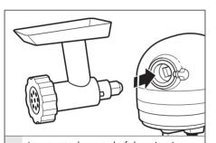
Insert attachment shaft housing into attachment hub, making certain that attachment power shaft fits into square attachment hub socket. It may 3 be necessary to rotate attachment back and forth. When attachment is in proper position, the pin on the attachment will fit into the notch on the hub rim.
