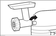
Tighten attachment knob by turning 4 clockwise until attachment is completely secured to Stand Mixer.
