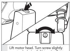
counterclockwise (left) to raise flat beater or clockwise (right) to lower flat beater. Make adjustment with flat beater, so it just clears surface of bowl. If you over adjust the screw. the bowl lock lever may not lock into place.
