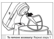
and 2. Press accessory upward 4 as far as possible and turn to the left. Then pull accessory from the beater shaft.
