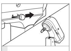
Hold the locking lever in the UNLOCK position and tilt motor head back.
