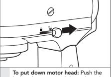
locking lever to UNLOCK and gently bring the head down. The locking 2 lever will automatically go back in LOCK position when the head is down. Before mixing, test lock by attempting to raise motor head.
