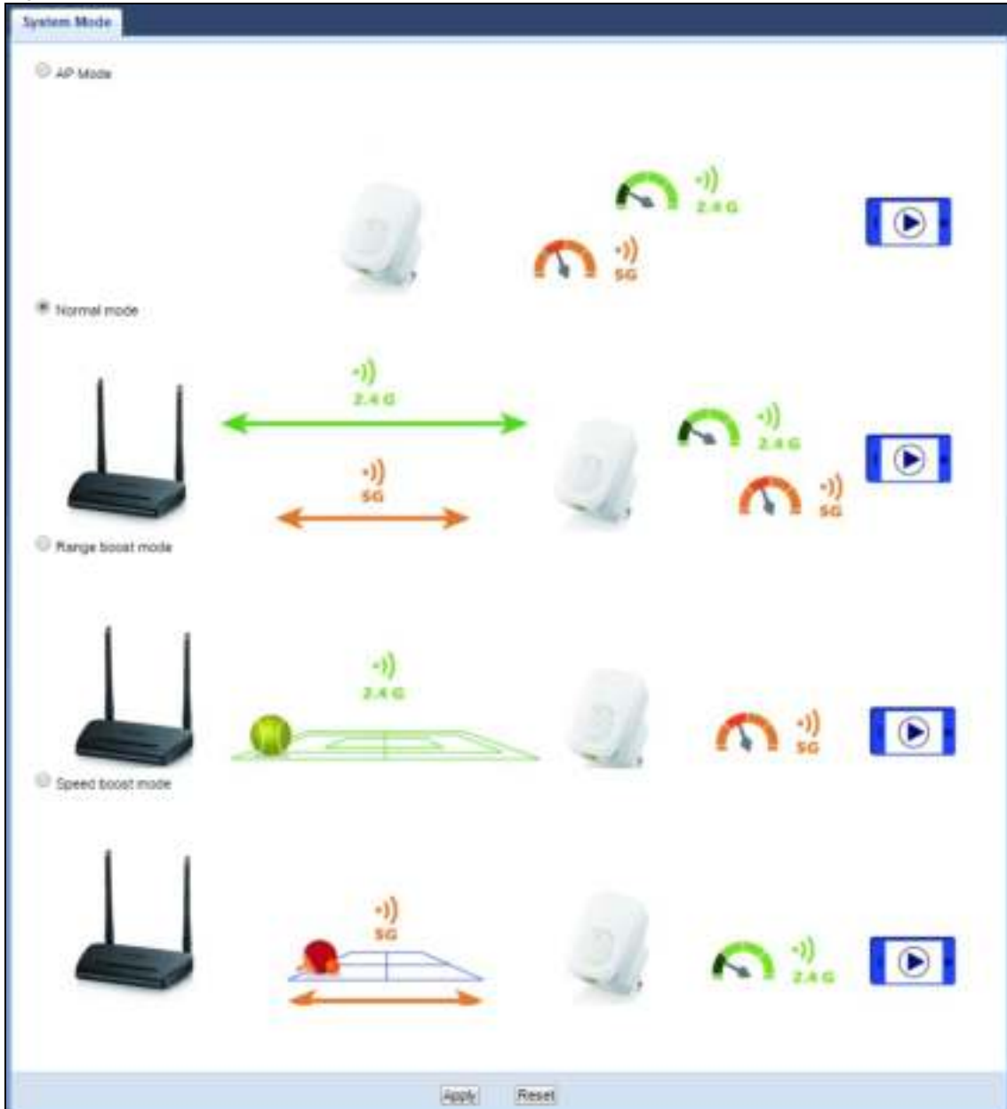
Figure 56 Maintenance > System Mode
