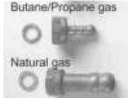
(2) In all cases, make sure the seal is fitted. Following the connection operations, test the leak tightness using soapy water, testing by flame is strictly prohibited.
