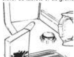
To add salt, unscrew the cap of the salt dispenser on the bottom and refill the dispenser.
