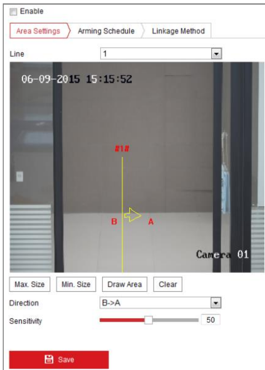
Figure 10-21 Line Crossing Detection
