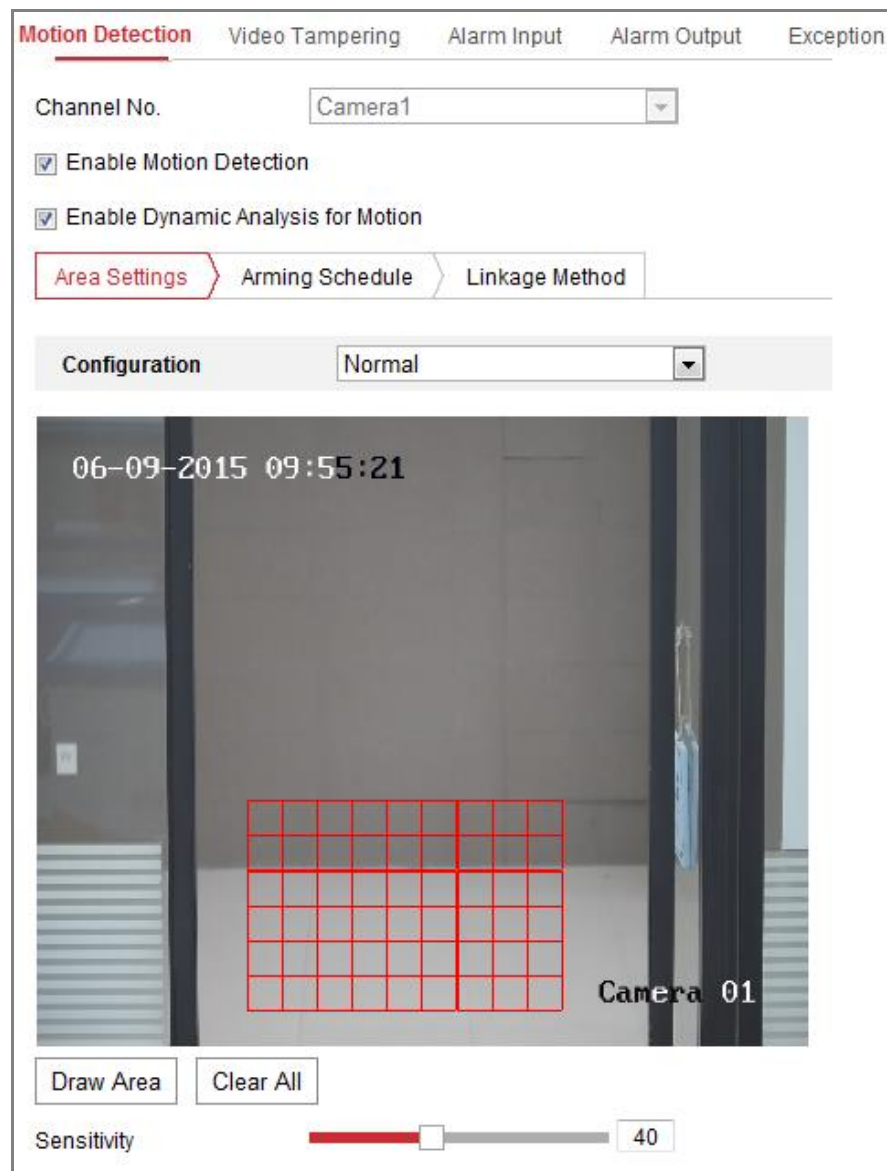
Figure 10-1 Enable Motion Detection
