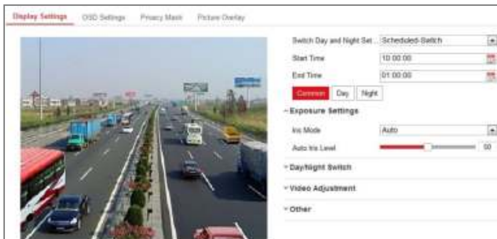
Figure 9-5 Day/Night Scheduled-Switch Configuration Interface
