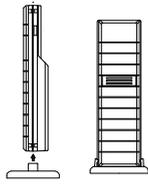
The Transmitter is supplied with a holder that may be attached to a wall with the two screws supplied. The Transmitter can also be position on a flat surface by securing the stand to the bottom to the Transmitter.
