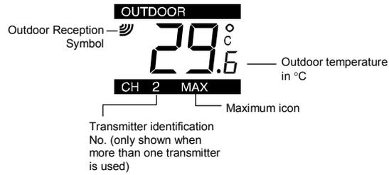
The last LCD section shows the outdoor temperature, a reception symbol and a channel number under the temperature will also show if more than one transmitter has been used.
