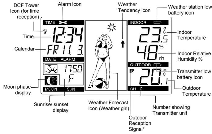
\*When the signal from the transmitter is successfully received by the Temperature Station, this icon will be switched on. (If not successful, the icon will not be shown on the LCD). User can therefore easily see whether the last reception was successful ("ON" icon) or not ("OFF" icon). On the other hand, the short blinking of the icon shows that a reception is being done at that time.
