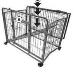
**5.** Secure the top of the cage by pushing the 2 locks through and turning the latches to the right.
