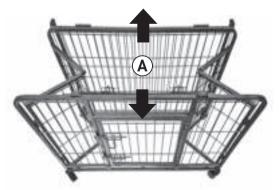
**3.** Push the folding parts together on both sides of the cage.
