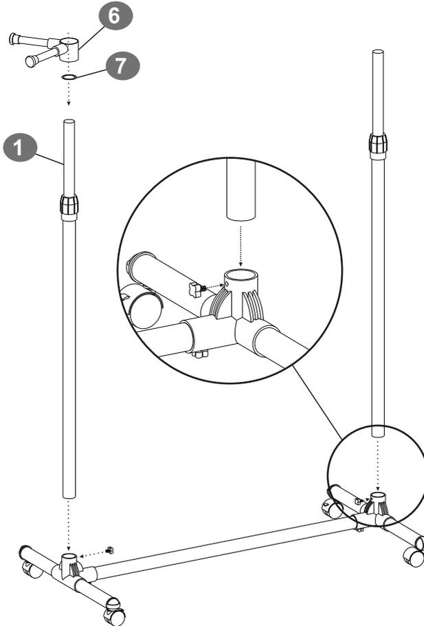
**EN** • Please make sure that the tubes have been inserted into the bottom of the plastic connectors.
