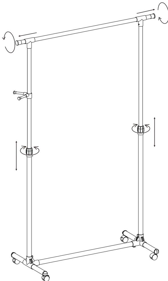
**EN** • Please tightening the plastic connectors after assembling or height adjustment.
