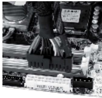
ATX 20+4 connector with 4 pin connector separated (left picture) and attached (right picture)
