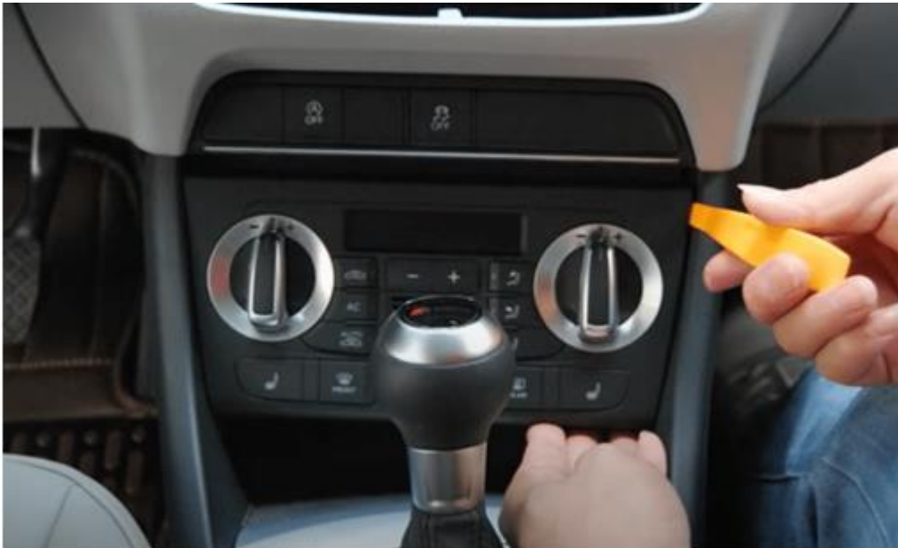
Audi Q3 climate control panel removal
