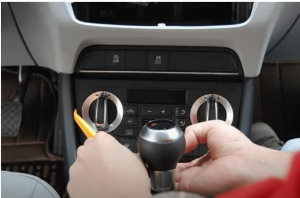
Audi Q3 climate control panel removal
