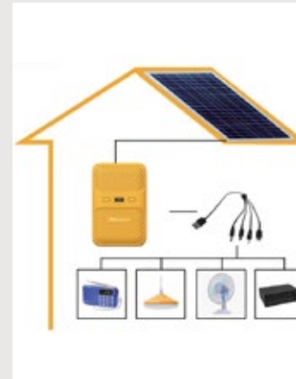
Solar home lighting system
