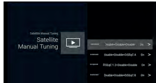
Satellite Manual Tuning: manually search for a certain TP, which can be added by Satellite Add if needed.
