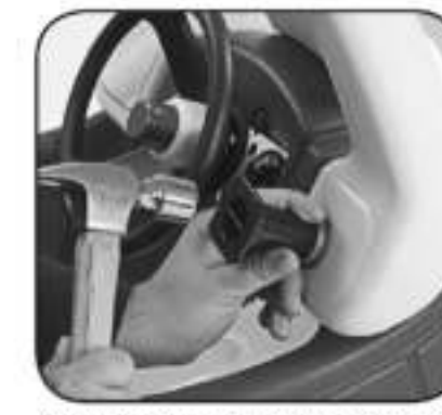
Place axle cap tool over ignition base and hammer. Snap on ignition top.
