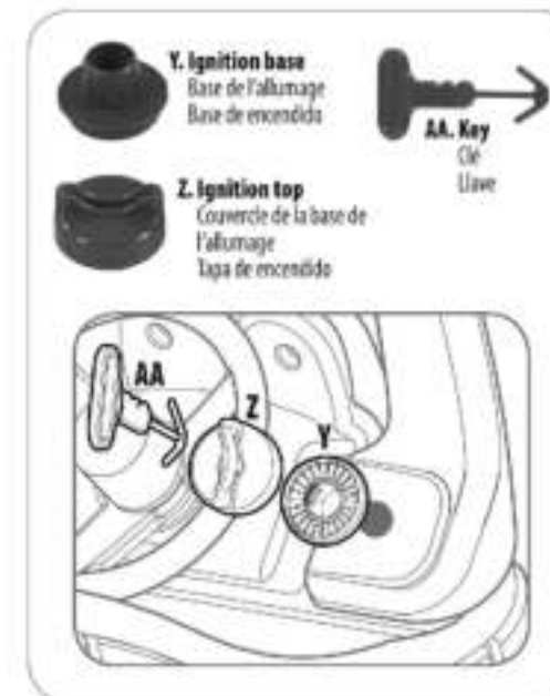
Place axle cap tool over ignition base and hammer. Snap on ignition top.
