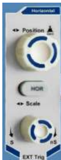
Figure 3-11 Horizontal Control Zone
