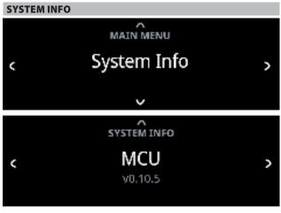
"System Info" displays information about current MCU, LCD and FPGA firmware versions.
