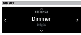
DIMMER function makes it possible to adjust the brightness level of the front panel display.
