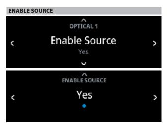
One can enable/disable a Source via this option. This is particularly useful if only few Sources are used thereby bypassing unused sources.
