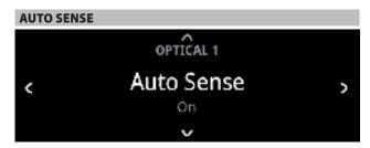
Auto Sense can be setup for each Source. Auto Sense feature enables the designated Source to wake up from standby mode when an active source is detected from the particular Source's input.
