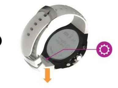
Remove LEDs Battery Clip
