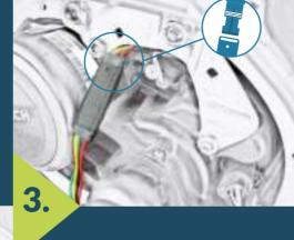
3. Couple display connector with BikeTrax connection cable
