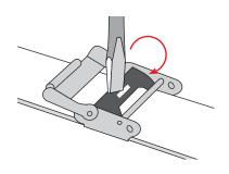
3. Insert the adjustment tool back into the slot and lock it down towards the strap.
