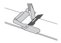
Open the top clasp. Insert the adjustment tool in the slot and lift it up.
