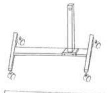
Step 2: Fix the four universal wheels to the I-heam and install the two wheels with brakes on the same side.
