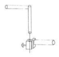
Step 3: Link the L-shaped steel pipe and the small steel pipe together with a handle
