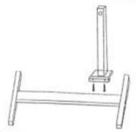
Step 1: Link the column and the I-shaped steel pipe with two 65CM long screws and nuts
