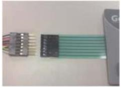
(If you connect the panel cable wrong way the red lamp on the panel will constantly light. It will not damage the product.)
