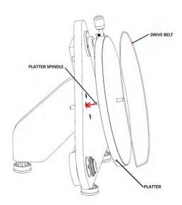
After placing the record on the platter, it is necessary to tighten the screw-able record clamp (6) onto the platter spindle.
