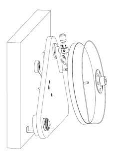
After the placing the record on the platter, it is necessary to tighten the screw-able record clamp (6) onto the platter spindle.
