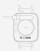
A Be aware that the two pins of the USB cable are not allowed to contact the conductor at the same time, or it will cause short circuit and burn.
