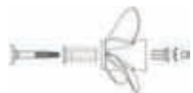
Fig. 8 The forward thrust washer MUST be installed first. Failure to install a forward thrust washer will cause gearcase damage and potential injury.
