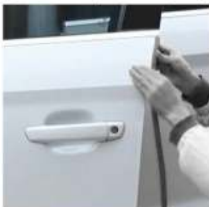
③ Use the tool to press the strip into place
