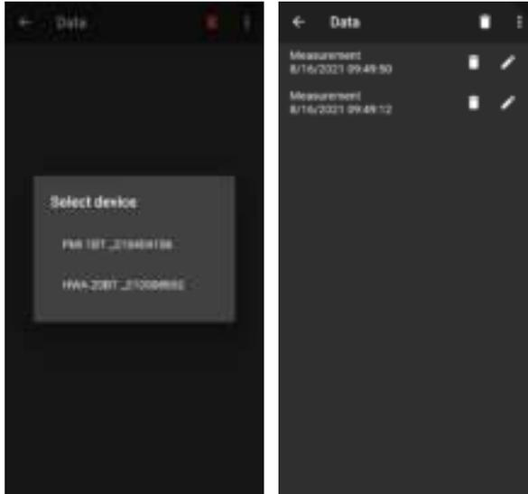
Each measurement can be renamed or deleted via the associated options. Furthermore, it is possible to view the measured values by tapping on the desired measurement.
