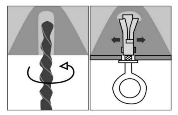
• Drill three holes in the ceiling (make sure there are no electrical wires or pipes in the ceiling), then fix the power line box to the ceiling. Pay attention to the distance between the wall to
