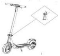
Using hex wrench in the packing box to tighten the screws on handle bar
