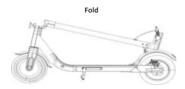
Make sure scooter be off , hold the front pole , loosen a lock lever and lower a steering rack . Adding a steering rack in a horizontal position and secure it by inserting a hook through a special ring , which is located on the rear wheel mudguard . To Assemble the scooter , disconnect a steering rack lock from a hook of a mudguard , and then lift it into a vertical position and lock a lever .
