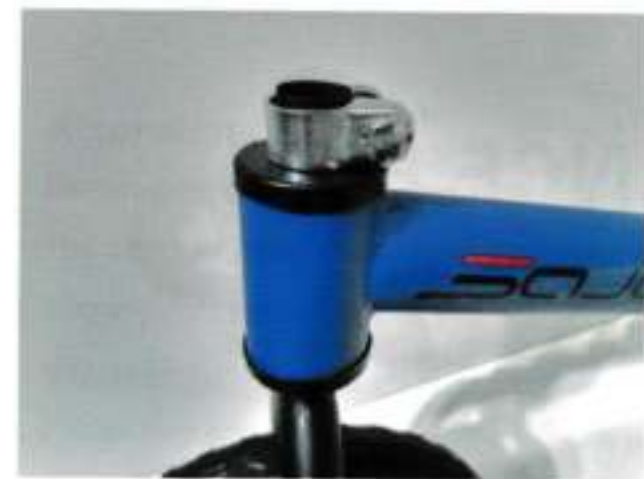
1. Place the steering wheel on the fork.
