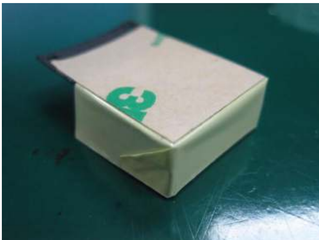
Picture 34 Insulator provided under L501 (GPS-1000DB XX)
