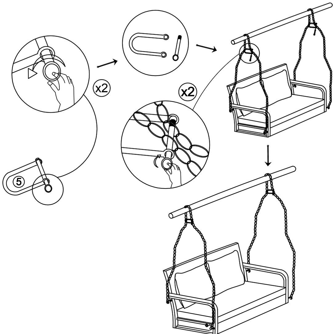
**Connect the part from step 5 & Lock (5) to finish.**
