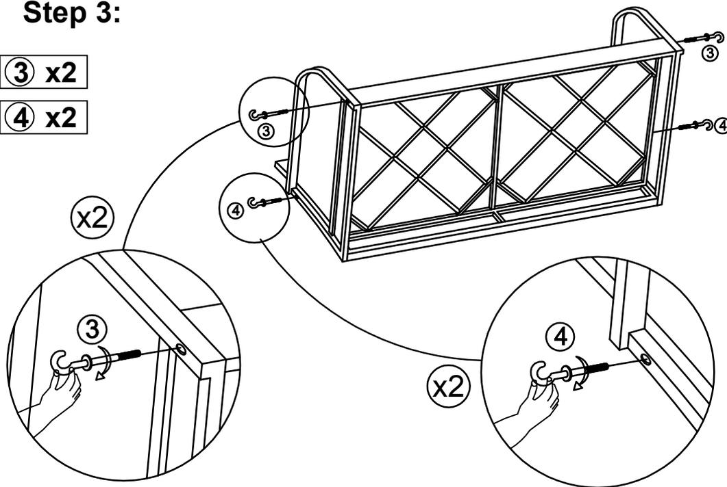
Connect the part from step 2 & tighten Hook (3) & Hook (4).
