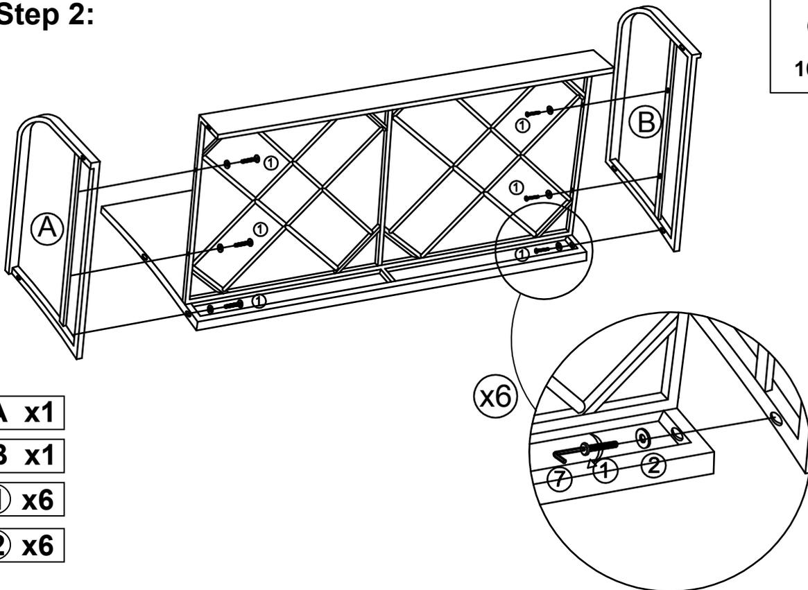
Connect the part from step 1 & Right Arm (A) & Left Arm (B), tighten Bolt (1) & Flat washer (2) with Allen Key (7).
