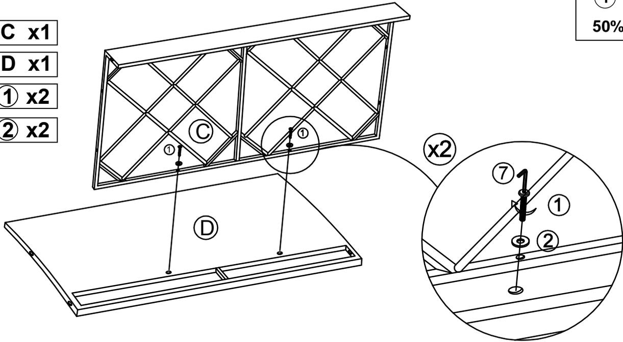
Push & Connect Seat (C) & Back Frame (D), tighten Bolt (1) & Flat washer (2) with Allen Key (7).
