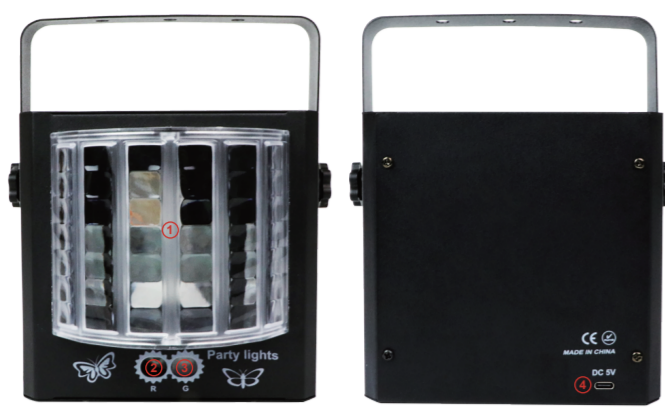
① LED light source ② Red pattern ③ Green pattern ④ DC 5V Input
