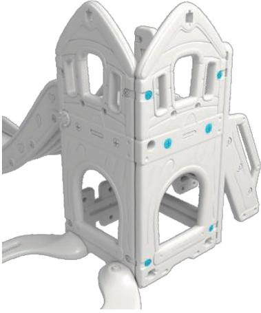
14. Connect the other side of bottom panel with castle side panel with Nut A and tighten with tool.
