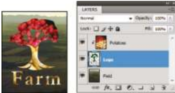
Clipping mask: content of the clipped layer (Potatoes) is only visible within the content of the base layer (Logo)
