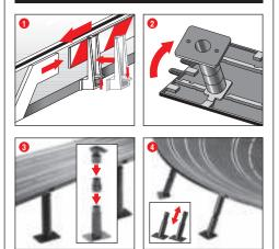
1 Guard rails: Guard rail mounts are fitted by tilting them upwards onto the verge of the track.
