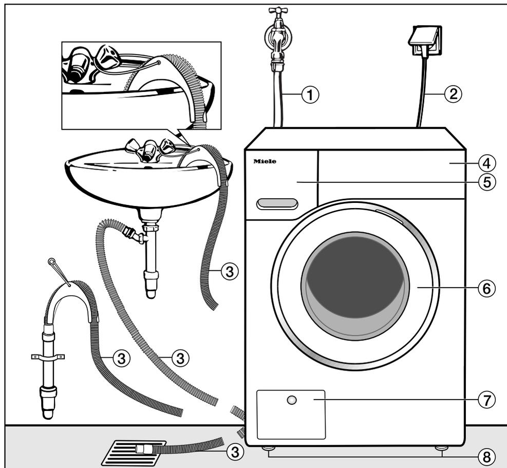
① Water inlet hose (pressure tested to 7000 kPa)
