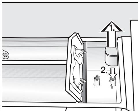
1. Remove the siphon from
