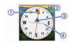
The course pointer ① indicates your relationship to the course line leading to the destination. The course deviation indicator (CDI) ② provides the indication of drift (right or left) from the course. The scale ③ refers to the distance between dots ④ on the course deviation indicator, which tell you how far off course you are.
