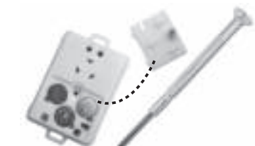
Insert or replace 3 button cell 1.5 volt LR44 batteries inside
