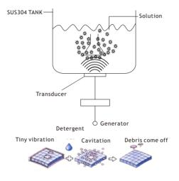
Ultrasonic cleaning is based on the cavitation effect caused by the vibration of high frequency ultrasonic waves in the liquid. Microscopic bubbles are formed. These implode causing the cavitation which create an intense scrubbing action on the surface of the item being cleaned. The bubbles are small enough to penetrate microscopic crevices, cleaning them thoroughly and consistently.
