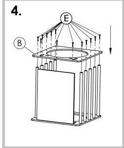
Note: - Use ALLEN KEY (D) to screw the SCREWS (E) into the predrilled holes.
