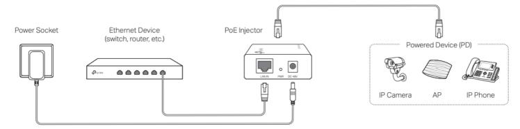
Note: The maximum output power of TL-POE150S is 15.4W. PoE devices that require more than 15.4W are not supported.
