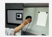
brightness and set it as the target value for calibration to ensure uniform brightness between your monitor and light box when color proofing.
