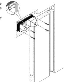
4 Along the wall, carefully cut off the unwanted part of box frame, do not damage the white upper cover whilecutting.
