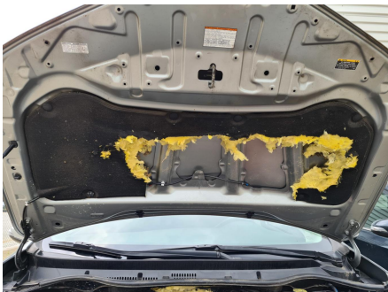
Example: Damage under the hood by a stone marten.
