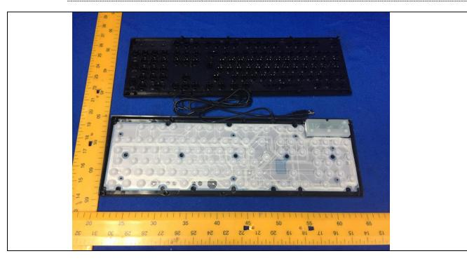
Internal view 1 of product after IP5X test Details of:
