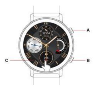
Button A: Long press to switch ON/OFF, short press to turn ON/OFF the screen.
