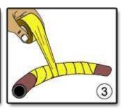
For high-pressure leaks, additional wrapping may be required. Most hose repairs can be repaired with 3-5 layers thickness, wrapping 3-5 inches in each direction away from the leak. Additional strength can be added by wrapping more Rescue Tape.
